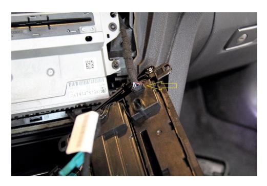
7. Remove the four indicated T-15 torx screws and set them safely aside. Gently slide the head unit forward to expose the cables on the rear. The unit is heavy, I recommend putting a shop towel over your lower dash to protect it.
