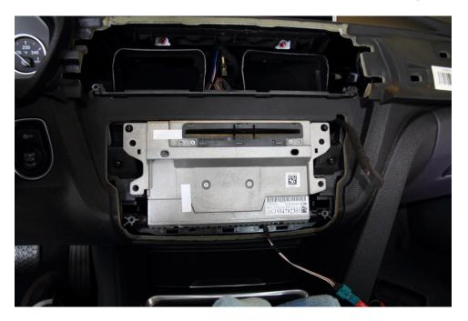
14. Double check your connections down from the screen, to make sure they are not wrapped up around the vents or pulled too tight. Plug the AC/stereo trim back in, and reinstall using the four T-15 torx screws. Also reinstall the cover below the AC/stereo controls. Secure the screen with the last two T-15 torx. Be careful to not overtighten the screws into the nylon sockets.
