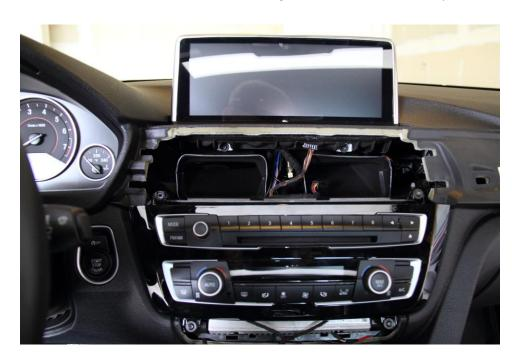
15. Connect both cables to the center trim, with both plugs being keyed so can only insert one way. Slowly press the trim piece back into place with gentle firm pressure. Also, gently press the trim all the way down to the right, until it is all fully in place.
