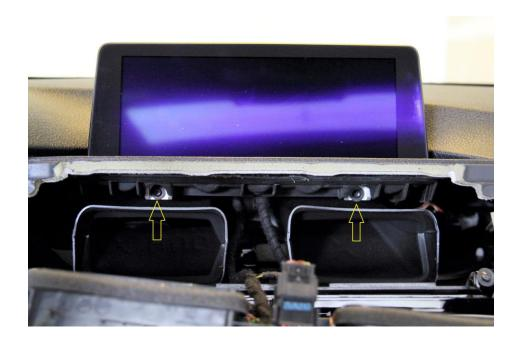
3. Press in the small tab marked by the arrow, and gently remove the plug by pulling straight out. You can also use a trim tool to *gently* pry under the plug to help guide it out. Set the screen aside.
