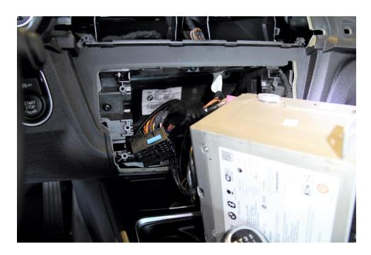
9. **Critical note:** The black and green optical cables need to be removed from the original plug and transferred to the provided adaptor or you will not have sound. Gently lift the indicated tab, and slide out the connector for the black and green optical cable. Install the optical cable in the matching position in the male plug of the provided adaptor cable. The plug is keyed and will only install one direction.
