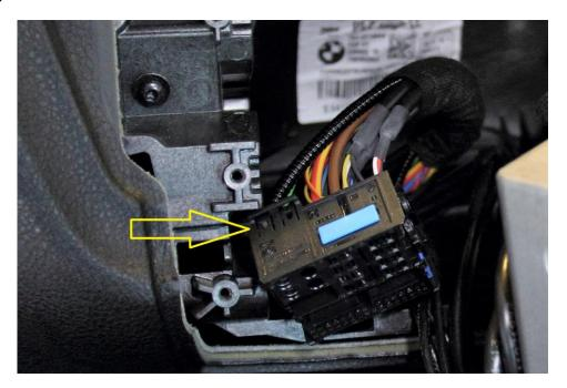
10. Insert the original male canbus cable into the female plug of the provided adaptor cable, and the male end into the head unit. **Important note:** I removed the cable wrap show in stage 9 around the wiring bundle, to give additional length to the optical cable for the new adaptor.
