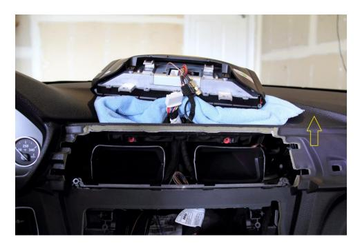
13. Double check all connections, and then slide the head unit back into place. It is easier if you get as much of the new adaptor cable and plug down into the lower right as you can first, before sliding the unit back. Don't force it to move, and remove and rearrange cables as needed to allow smooth installation. Secure the head unit with the four T-15 torx when in place.
