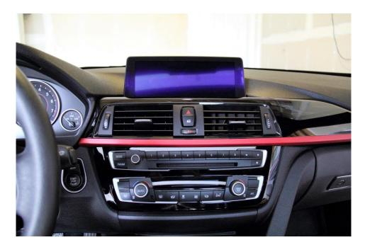
2. Remove the two exposed T-15 torx screws to free the screen, and gently pull up and turn to expose the cable connection. Slide a little extra cable up if needed to get it higher to turn.
