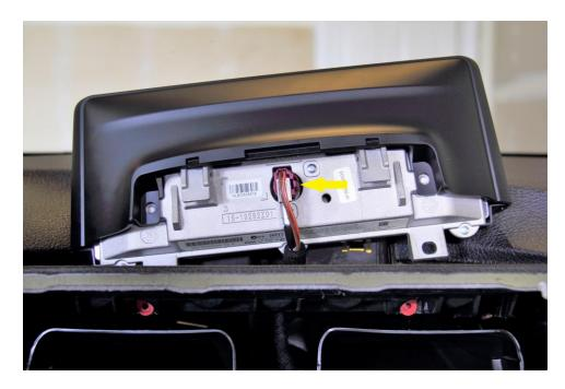
4. Remove the two indicated T-15 torx screws, and remove the dash cover below the AC controls. Remove the cover by gently pushing in and down just below the controls.
