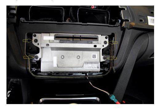
8. Remove the large black canbus connector from the head unit. This plug is in the center of the head unit, and has a horse collar connector. Gently pull back the collar, and the plug will unlock and walk back out of the connection.
