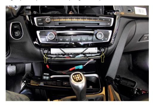
6. Remove the single indicated plug, to free the AC/stereo piece and give extra room to work. Be gentle removing this plug, it can be very hard to remove in some cases. Set the piece aside.
